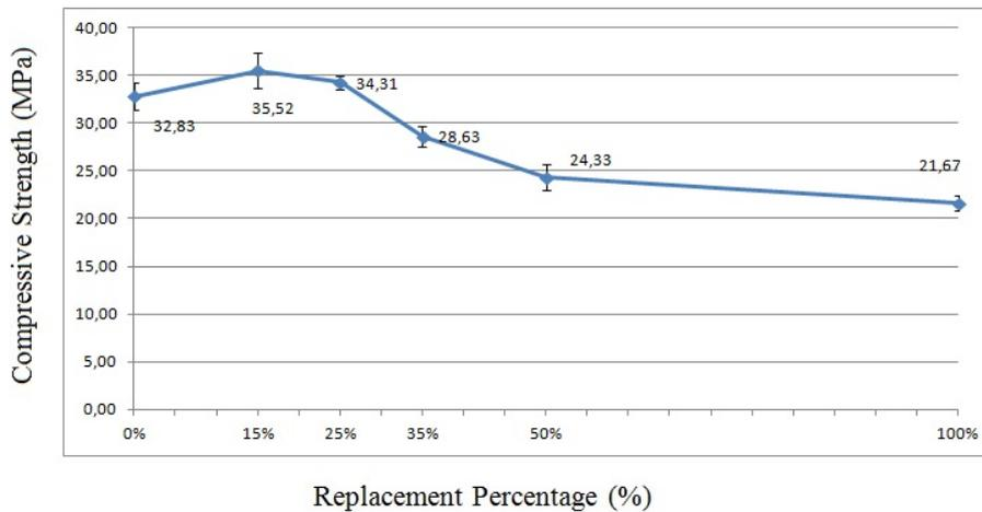
Figure. 2 Effect of recycled aggregates on 28-day compressive strength.
