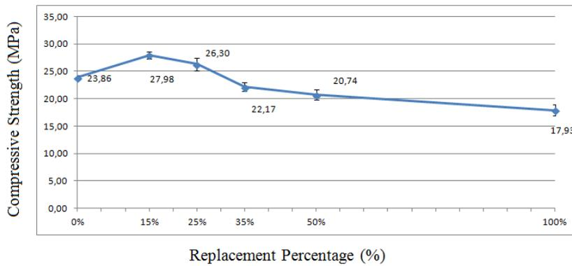
Figure. 1 Effect of recycled aggregates on 7-day compressive strength.
